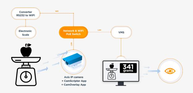
This demonstration shows how easy it is to enter data directly into the camera image. No computer or server is necessary – everything happens inside the camera. The digital scale is only an example of the many things that can serve as a source of data. The micro application in the CamScripter App can easily send data or events to another system.
